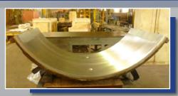
ALC specializes in the redesign and improvement of drive and slide shoe bearings. ALC owns many patterns and has extensive references of drive and trunnion bearings.
